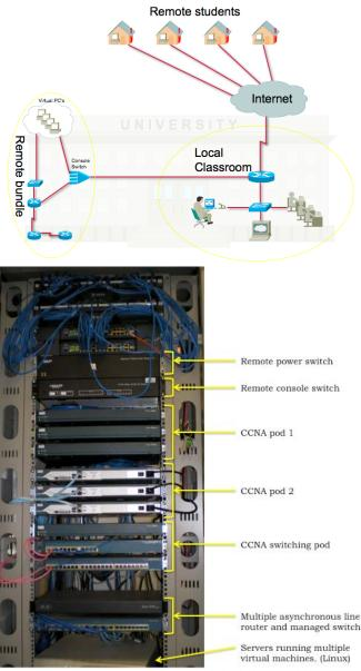
Figure 3: Teaching environment (top) and physical remote laboratory equipment layout (bottom)
