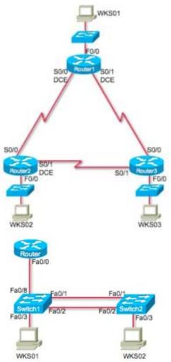
Figure 2: Standard router bundle (top) & Switch Bundle (bottom)
