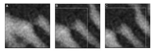
Corresponding series of images fed to the DSP for processing. The white lines mark the overlap with the previous image.
